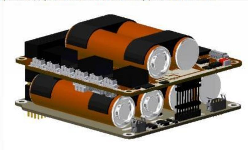
Stacking height between the P31u and BP4 PCB is 23.5mm.
