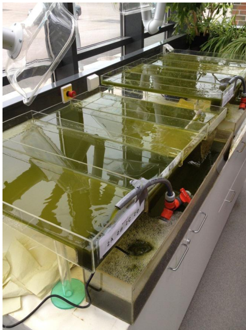
Figura 8: Tanques “Turf Scrubber”.
