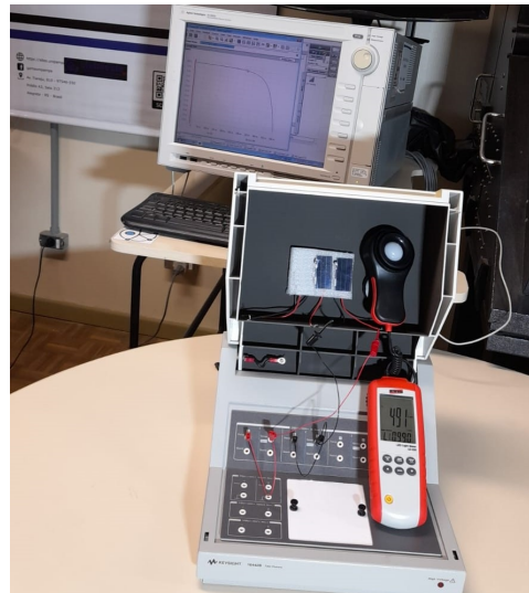
Figure 23 – Experimental setup for the PV cell I-V measurement.
