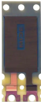
Figure 9 – Piezoelectric Generator PPA-1014.
