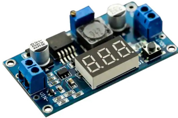
Figure 3 – Common buck-converter module.
