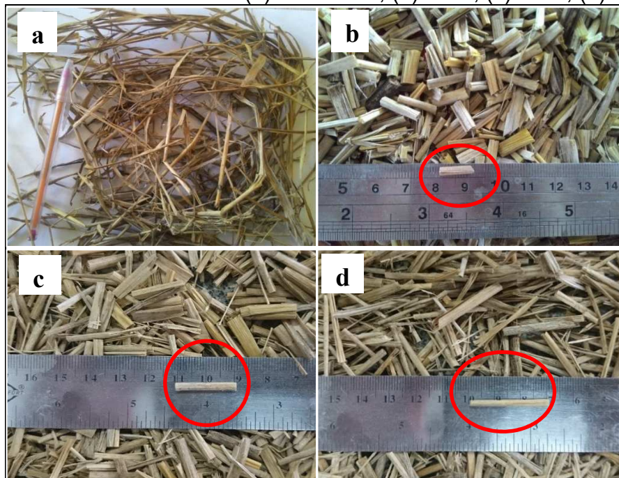
Figura 20 – Palha do Arroz: (a) “in natura”; (b) 1 cm; (c) 2 cm; (d) 3 cm;
